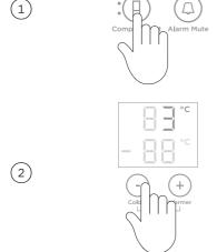
Press a until the refrigerator compartment light is illuminated, indicated by the top light.
