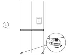
Wind up the feet and carefully ease the refrigerator out of its position. Switch off and unplug.
