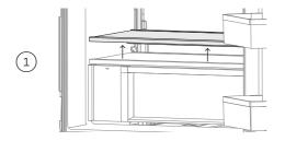
Lift the shelf up vertically. The Humidity Control Lid is attached to the shelf and will be removed together.
