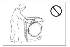
Never place cardboard, wood or similar materials under the machine to compensate for any unevenness in the floor. Install the machine on a flat hard floor. Make sure that air circulation around the machine is not impeded by carpets, rugs etc.
