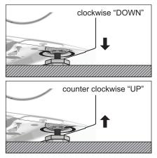
When the Washer-Dryer is levelled, try to rock it from corner to corner. If it does rock, adjust the legs again until it is levelled and does not rock.
