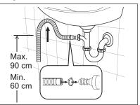
Push the drain hose onto the spigot and secure with a clamp, ensure a loop is formed in the drain hose to prevent waste from the sink entering the appliance.
