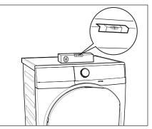
If you do not have a spirit level, as a guide use the edge of a door frame, cupboard or bench to check that the machine is leveled. Loosen or tighten the feet to adjust the level. A correct adjustment of the appliance level prevents vibration, noise and the movement of the appliance when in operation.
