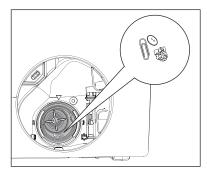
6. Make sure that the impeller of the pump can turn. If this does not occur, contact the service centre.
