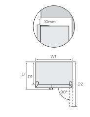
When positioned in a corner area, clearance of at least 350mm on the fridge side and 250mm on the freezer side will allow the doors to open enough to enable the removal of the bins and shelves.
