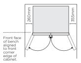
n a corne In a corner position, at least 355mm clearance on th' right hinge side and 260mm or the left hinge side will allow the doors to open enough to enable the removal of bins and shelves.
