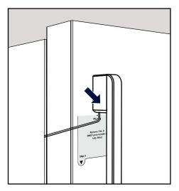
4 Lock the handle in place by FIRMLY tightening the screw using the SHORT END of the provided Allen Key.
