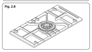
If, when you let go of the control knob the burner goes out, then the FSD has not been bypassed. Turn the control knob to the **OFF** position and wait for one minute before you try again, this time making sure to hold in the control knob for slightly longer.
