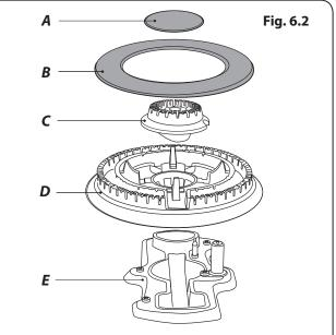
A – inner burner cap, B – outer burner cap, C – inner burner head, D – outer burner head, E – wok burner base
