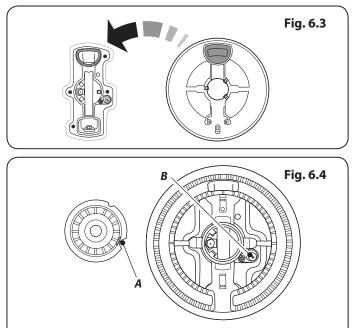
A – electrode notch, B – ignition electrode
