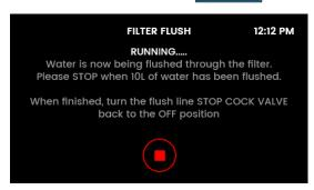
Stop flush, coil up flush line, close flush line tap.
