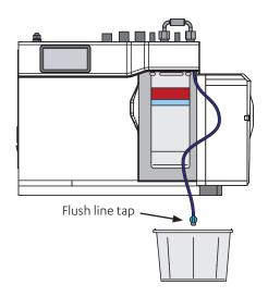
Open filter door, uncoil flush line.
