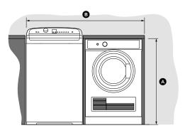
Note: Riser height 65mm (to be manufactured and fitted by a cabinetmaker)
