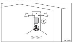
The silencer needs to be positioned between the exhaust connection and the directional unit ②. Ensure there is adequate space in the tower for fitting it.
